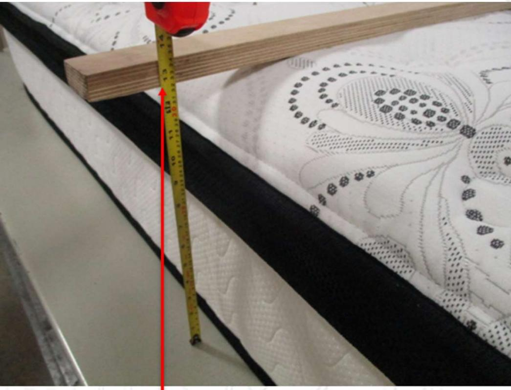
Measurement is to be taken at bottom of straight edge.
